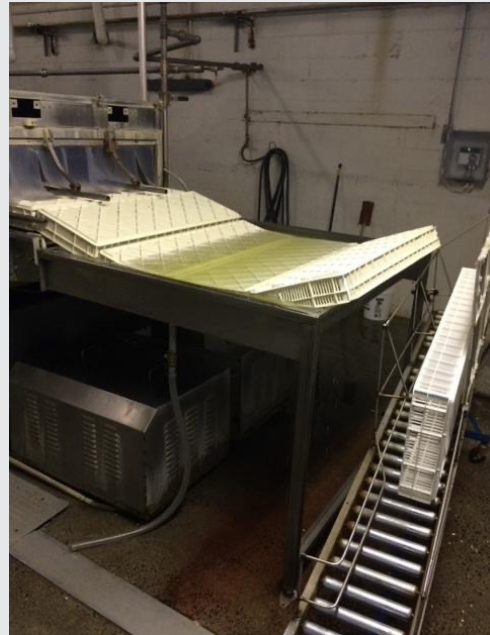
Figure 2a (left). Stainless steel disinfectant dip tank with a stacking belt assistant separating the employee from the warm temp and overspray.
