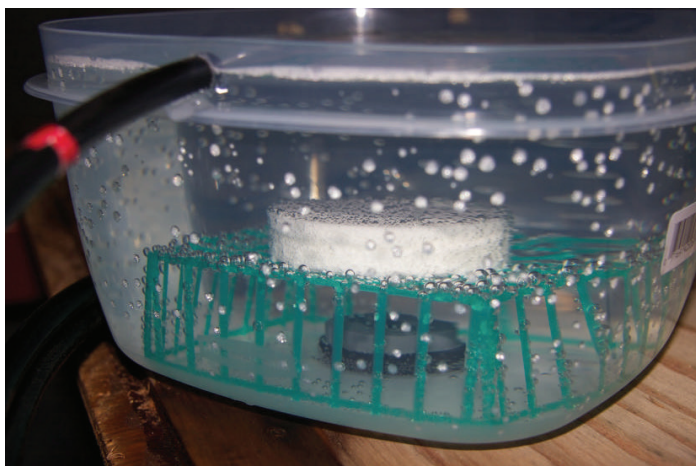
FIGURE 5 Detail of dissolution test apparatus
