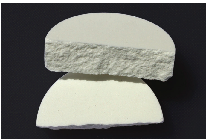
FIGURE 11 Detail showing the fracture surface of the tablets after a typical three-point bend test.
