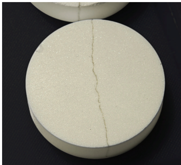
FIGURE 12 Fitting the tablet halves back together after the test shows how little material was lost as powder or splintering during the break
