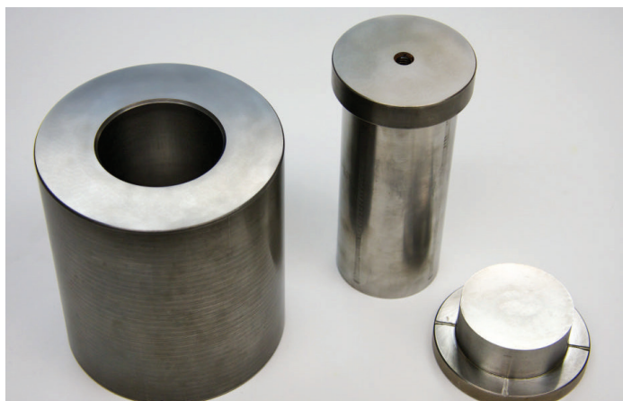
FIGURE 1 Custom-made stainless steel 2.5" punch and die set.
