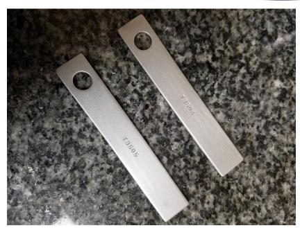
Figure 1. Mild steel coupons prior to contact with Peraguard.
