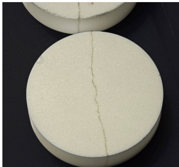
FIGURE 12 Fitting the tablet halves back together after the test shows how little material was lost as powder or splintering during the break.
