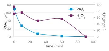
**Graph 1** illustrates the instability of PAA and  $H_2O_2$  on the surface of tomatoes. After 30 seconds the initial concentration was at 74.4 ppm PAA and 93.85 ppm  $H_2O_2$ . Over time, the concentration of the PAA and  $H_2O_2$  decreased gradually. After 90 minutes, the study was terminated due to the depletion of PAA and  $H_2O_2$  to a non-detectable limit of the instrument.
