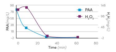
**Graph 2** illustrates the instability of PAA and H2O2 on the surface of yellow squash. After 10 minutes the initial concentration declined from 87.74 ppm PAA to at 30.74 ppm PAA and 137.58 ppm  $\rm H_2O_2$ . After 30 minutes, the concentration of the PAA measured below the detection limit of the instrument and the  $\rm H_2O_2$  decreased to 8.91 ppm. After 60 minutes, the study was terminated due to the depletion of PAA and  $\rm H_2O_2$  to a non-detectable limit of the instrument.
