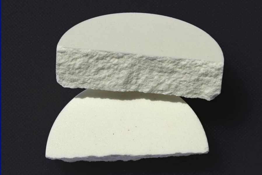
Detail showing fracture surface after a 3 point bend test.
