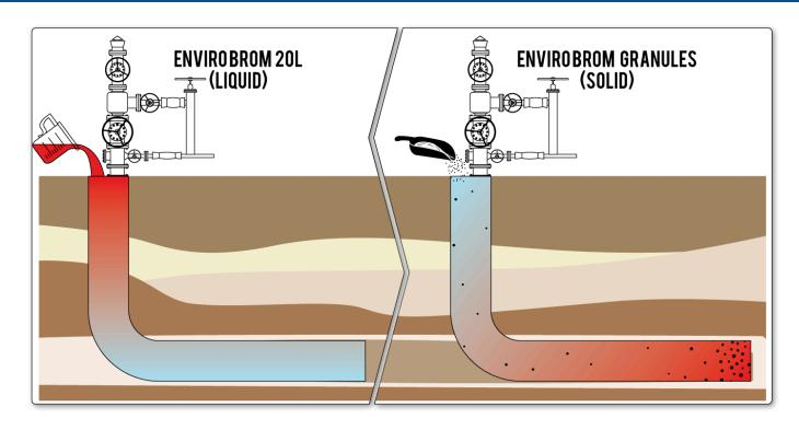
With liquid DBNPA, the region of highest concentration is near the surface.
