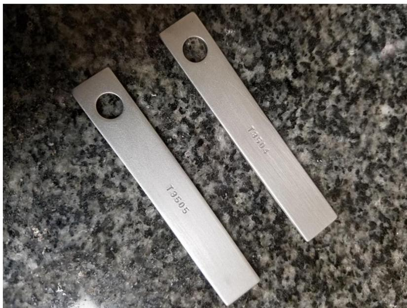
**Figure 1.** Mild steel coupons prior to contact with Peraguard.
