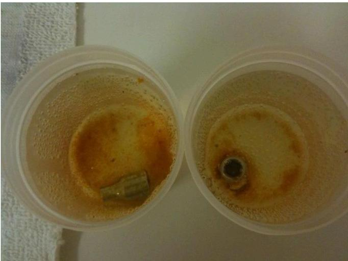
Although the solution of both the low grade chrome socket and high grade chrome socket turned to an orange-brown color throughout the seven day experimental period, only the low grade chrome socket showed signs of corrosion on the chrome plating itself, after the first day and continued to worsen throughout the seven day period.. The chrome plating covering the outside of the high grade chrome socket remained intact for the first part of the experiment but by Day 7, one small
