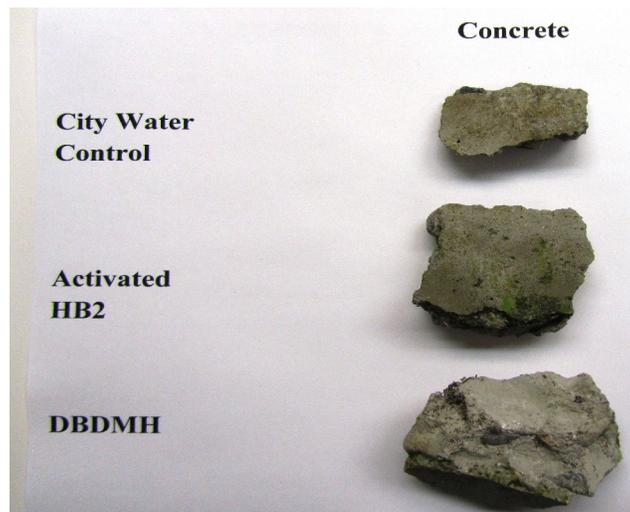
Similarly, the concrete pieces exposed for 30 days to both sources of HOBr appeared identical to the concrete exposed to the city water control. None of concrete pieces had lost any weight during the exposure period. Microscopic examination of the surfaces revealed no signs of etching or other damage. This is not surprising because both sources of HOBr are solutions that are close to pH neutral. There is no erosion or loss of weight for either DBDMH or liquid hypobromous acid.
