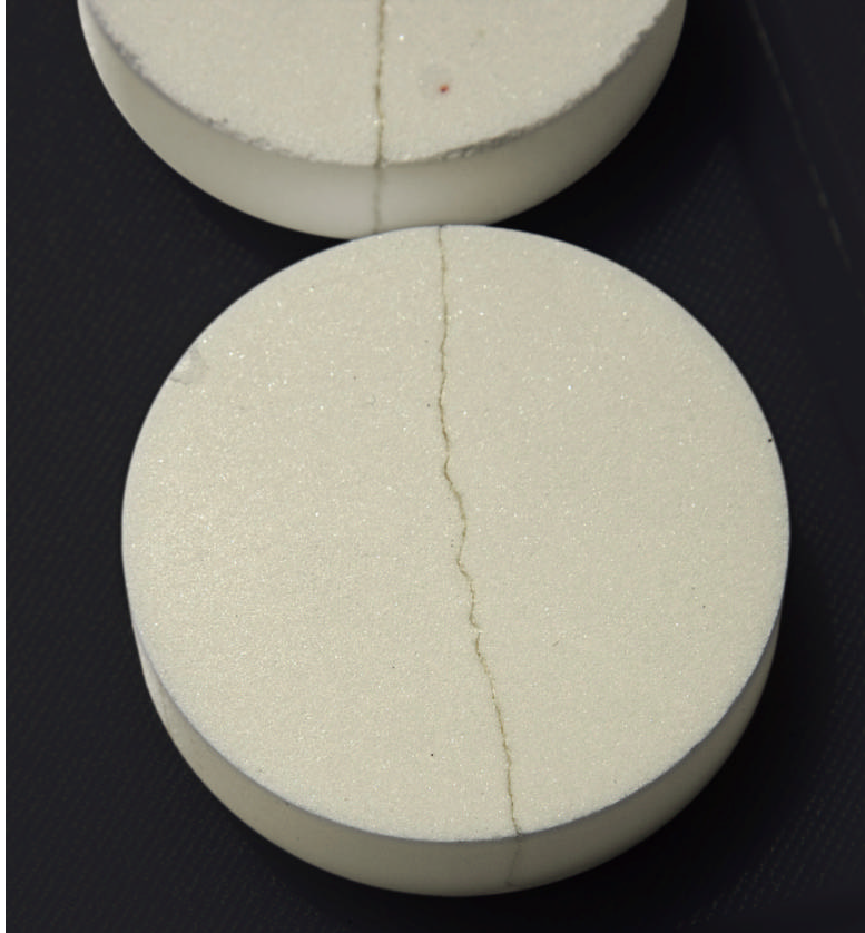
Figure 12 Fitting the tablet halves back together after the test shows how little material was lost as powder or splintering during the break.
