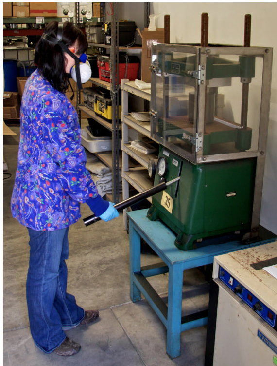
Figure 2 Carver Press Model 2626 being used to compact DBNPA crystals.
