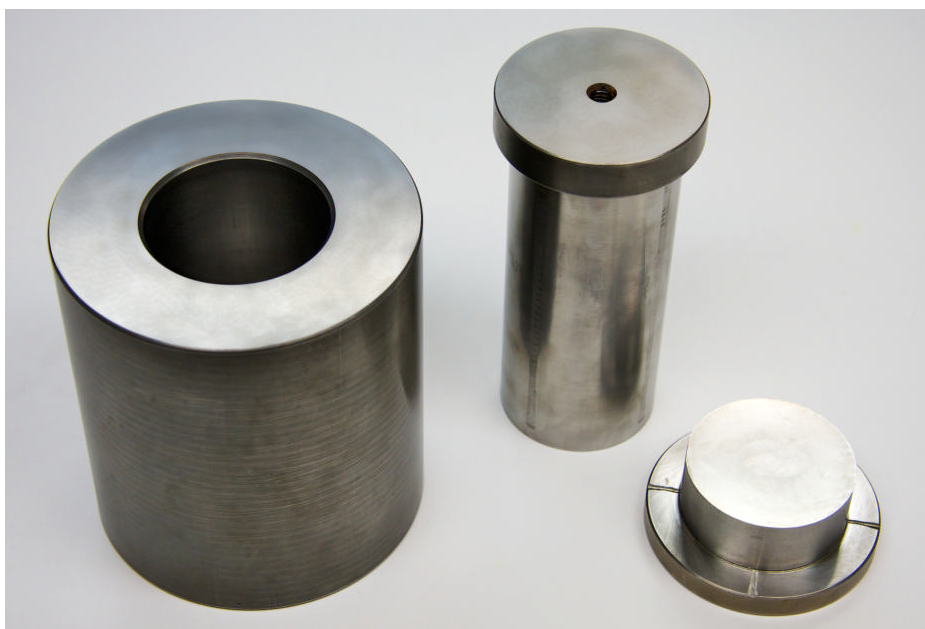
Figure 1 Custom-made stainless steel 2.5" punch and die set.
