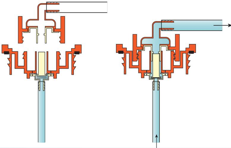
Internal spring-loaded valves only allow product to flow when mated with the appropriate Safe-T-Feed<sup>®</sup> tubing adapter.
