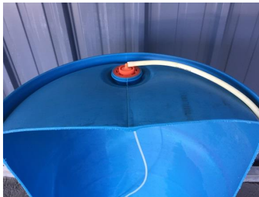
Safe-T-Feed dip tube and female adapter assembly.
